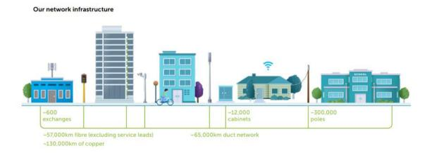
The Chorus Group's fibre or copper cables typically connect to local rural or urban exchanges, of which it has approximately 600 nationwide at the date of this Information Memorandum. The methods of connection from a premises to a local exchange are discussed further below.
