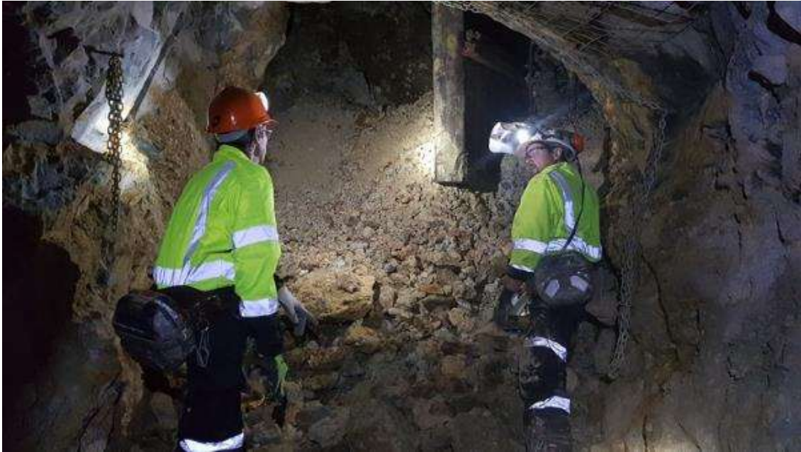
Figure 2 - the Brow of the Dubbo Rise showing fine material being loaded out
